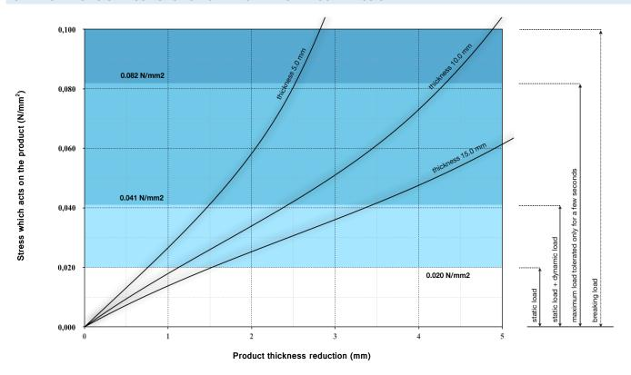
NOTE: Stress/Deformation analysis of the subfloor systems/dampers product, characterizes the own mechanical properties. The shape factor suggests the optimal load condition as the product can be subjected.
