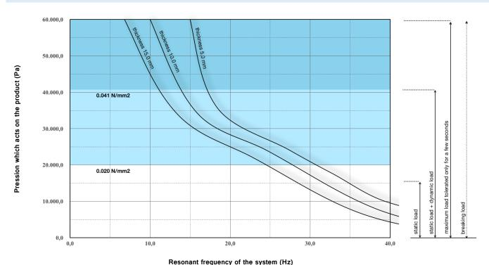
NOTE: System's resonance frequency and shape factor in relation to the different type of thickness.
