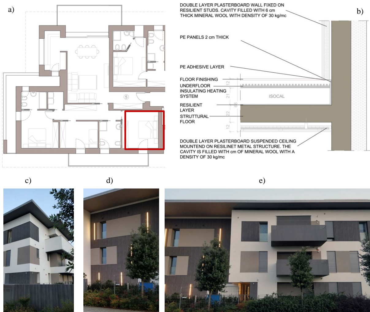
Figure 1: a) plan view of the apartment (in red the receiving room); b) measured floor; c), d), e) photos of the building.
